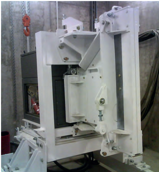
6 MeV Varian linear accelerator and its collimator
