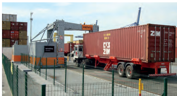
Relocatable linear accelerator used for inspecting loads
