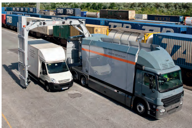
Mobile linear accelerator used for inspecting loads
